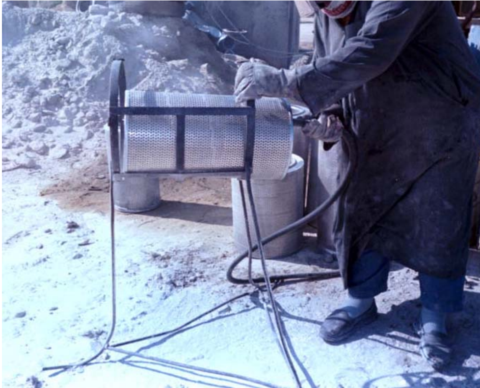
Cleaning of Air Cleaner Element
