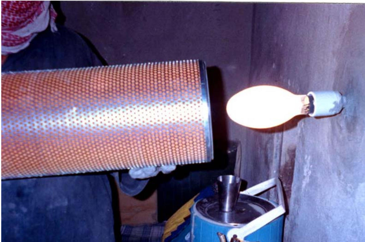
Checking Element for crack/torn paper
